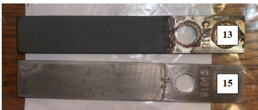
Figure 3.3.4 Two examples of the coupons after the month-long exposure experiment in Postgate-C. Sample 13 (top) was submerged in the non-RhL solution while sample 15 (bottom) was submerged in the RhL solution.
