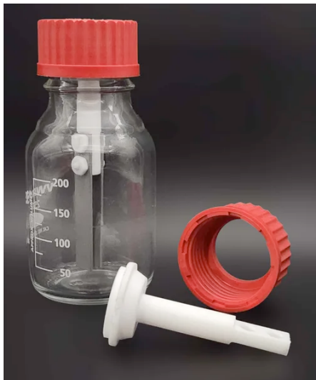
Figure 2.3 The deaeration set-up used 30 day immersion tests. Threads were sealed with PTFE tape and the cap was covered with parafilm.
