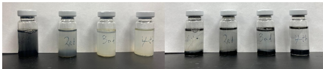
Figure 3.3.2: Inoculated commercially purchased “bug bottles” for detecting SRB activity. Left, as inoculated and Right 24hrs after inoculation showing production of sulfide in 3 rd and 4 th bottles.
